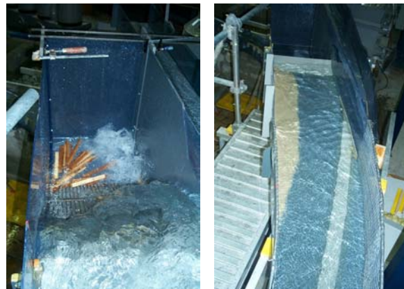
Fig.4 : Test with floating debris on the trash rack (left) and with sediment deposits upstream of the weir (right)
