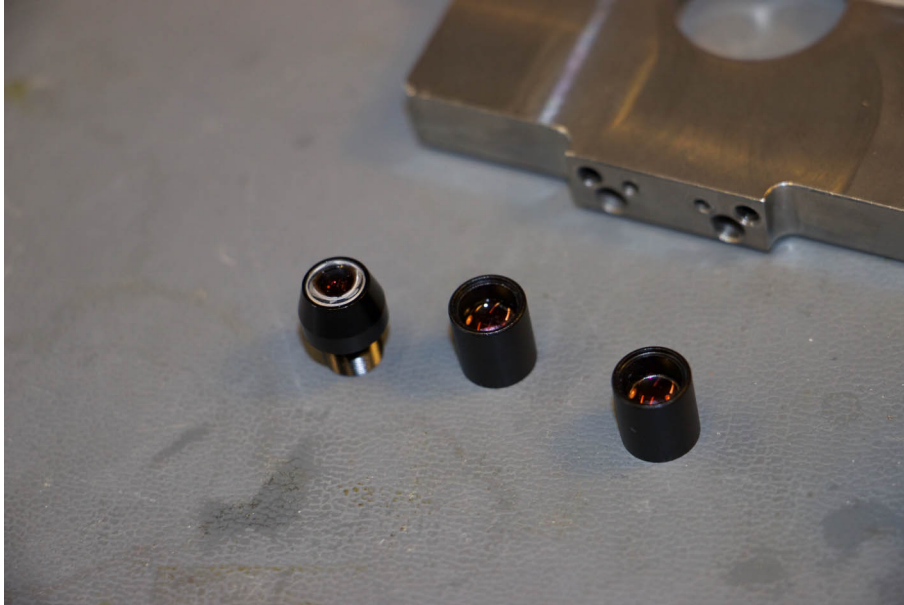
Figure 31: Glue the aspheric lenses into the objective holder and two collimation housings . All the lenses are Thorlabs A390-A . Put a very small amount of glue (2-tonne epoxy works well, a UV-curing glue could also work nicely) into the part where the lens will sit, and then drop the lens in. Avoid touching the surface of the lens or getting any glue onto the lens surface, it becomes very hard to clean afterwards. Keep things very clean as you work. Make sure the lenses are all sitting nice and flat. Refer to assembly technical drawings for orientation of the lenses if you're unsure.
