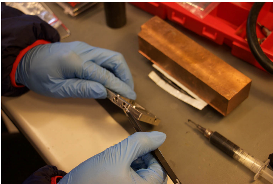
Figure 7: The translation stage middle guide gets held in place by the two 3 mm steel balls that were glued in in the previous step, and two 2.5 mm steel balls that are held in place by two compression springs (Gutekunst Federn model D-042F-03 ) and two 3 mm flat end set screws (4 mm length could also work). First ensure that the surface of the translation stage bottom plate upon which the translation stage middle guide slides (including the 3 mm steel balls ) is clean and greased lightly. Set the translation stage middle guide in place and hold it with a finger. Drop the greased 2.5 mm steel balls into the tapped M3 holes in the back of the translation stage bottom plate , followed by the D-042F-03 springs, and the 3 mm set screws with some thread lock. Tighten the screws until there is a significant restoring force on the translation stage middle guide , but that it still slides easily.
