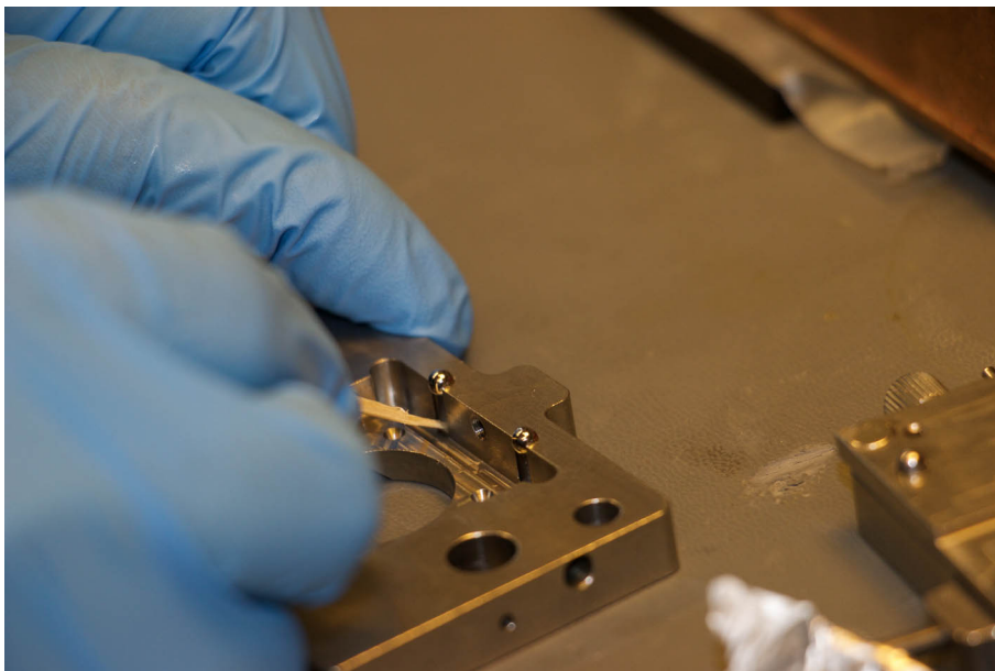
Figure 3: Place a small amount of epoxy glue (2-tonne is best) into the bottom of the holes in the translation stage bottom plate with the 3 mm steel balls placed at the top of the hole.
