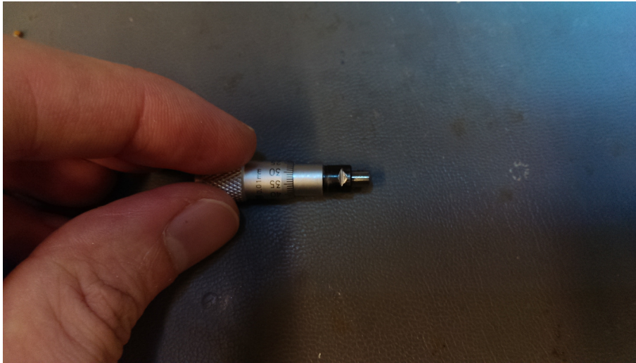
Figure 54: In another micrometer head (Thorlabs part no. 148-205ST-H ), cut a V-groove using a file or mill. The proper position of the groove can be marked by placing the micrometer head into the head housing hole for the focus micrometer and marking with a sharp object through the set-screw hole.
