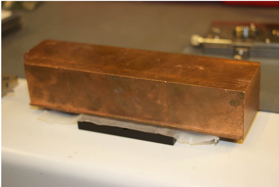
Figure 17: Clean up as much excess glue as possible, then wrap the corners in Parafilm and place the base plate onto a flat surface with a large flat weight to press the magnets in place while the glue cures.
