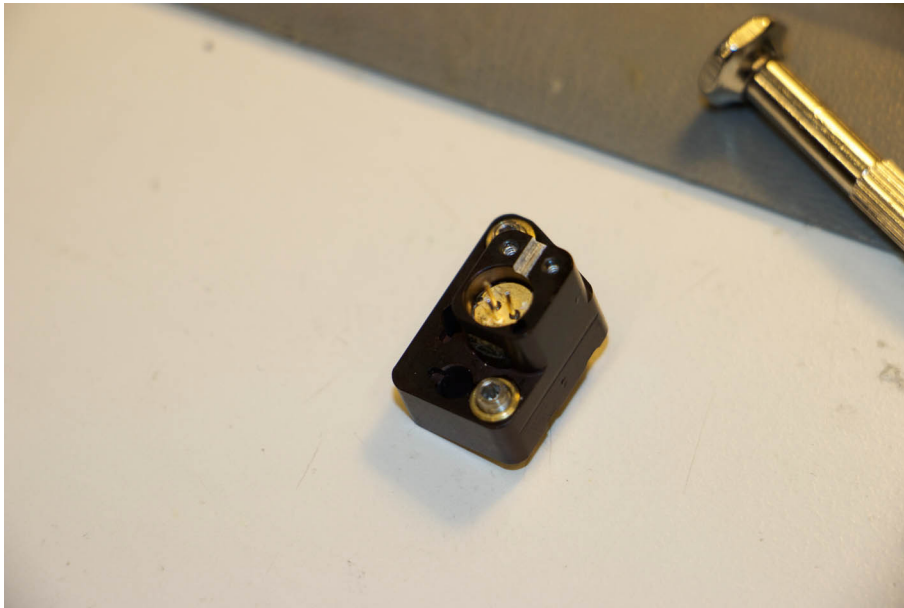
Figure 39: Glue in the Kozak Micro M3 matched thread/bushing pairs into the pt optics kinematic mount using 5-minute epoxy or equivalent. Put into the pt optics kinematic mount the collimated drive laser diode assembly in the correct orientation and tighten in place with an M3 set screw .
