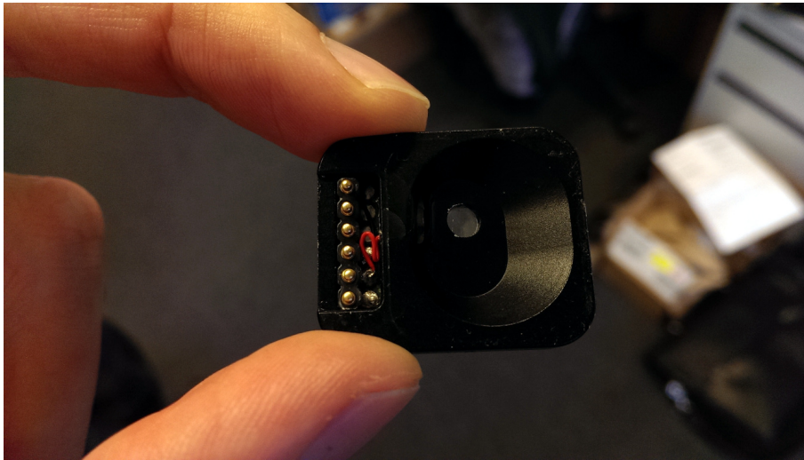
Figure 27: Glue in the cantilever holder PCB with superglue. Stack 2 copies of the 0.8 mm thick cantilever holder PCB under another one with the 6-pin spring mount electrical connector to get the right thickness (the part was designed for a different thickness PCB than was manufactured). Solder the leads of the 2x2x2 piezo to the appropriate pads as shown in the picture. Keep the leads as short as possible.
