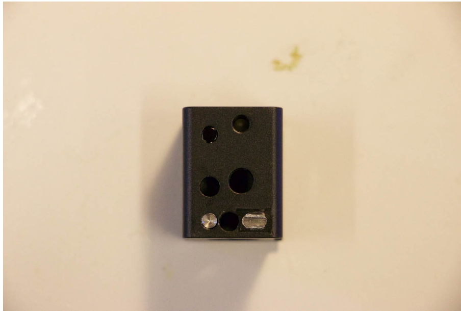
Figure 35: Glue in the 2.5 mm diameter sapphire window , the pt cone insert and the pt slot insert into the pt optics housing . 5-minute epoxy or equivalent is ok. The pt cone insert and the pt slot insert can be somewhat difficult to insert and may require the use of a vice or press. Make sure they are inserted straight. You can also glue on the optics bushing in the hole in the bottom of the pt optics housing at this stage as well.
