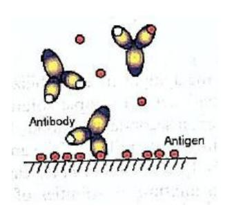
Sensor preparation: The target antigen is immobilized on the sensor surface.
