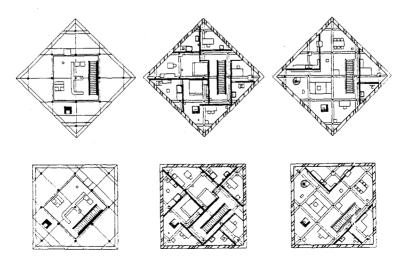
"When a diamond form in plan is projected by isometric it becomes a square. (...) The converse has been in existence and use, that is, the square drawn in isometric which becomes a diamond.
