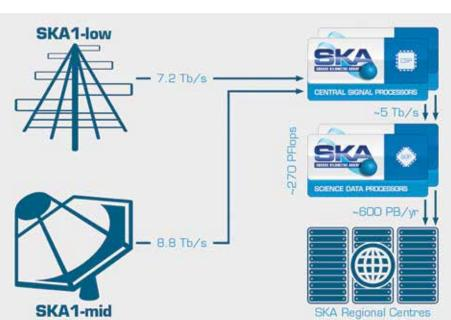
Figure 30 Data transfer rates between the SKA telescopes, processing facilities and regional centres. Credit: SKA Technical Paper (January 2019)
