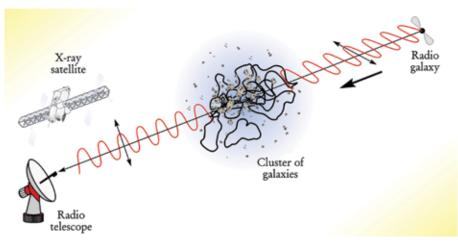
Figure 13 Illustration of the Faraday rotation effect in the magnetic field of a galaxy cluster observed by a radio telescope. The galaxy cluster is observed independently by X-ray satellites. Credit: Philipp P. Kronberg, Physics Today, December 2002, p. 40. Copyright 2002, American Institute of Physics
