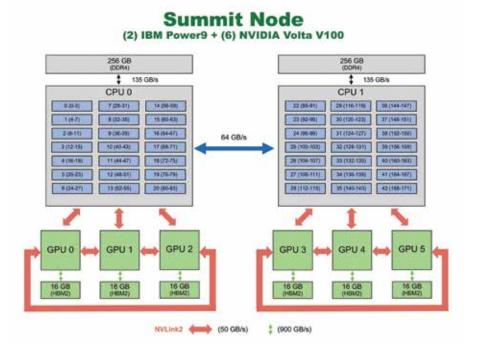
Figure 38 The hybrid computing node of the Summit supercomputer at the Oak Ridge National Laboratory in the USA, ranked N.1 in the TOP500 list on November 2018. Credit: Oak Ridge National Laboratory
