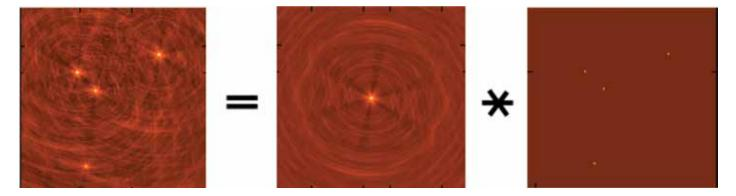
Figure 32 The RI data (left) expressed as the convolution of the dirty beam (middle) with the sought image (right). Credit: casa.nrao.edu
