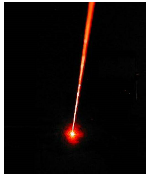
1970 1 st laser diode \lambda \sim 780 \text{ nm} J_{thr} \sim 4.3 \text{ kA/cm}^2 Ioffe, Russia
