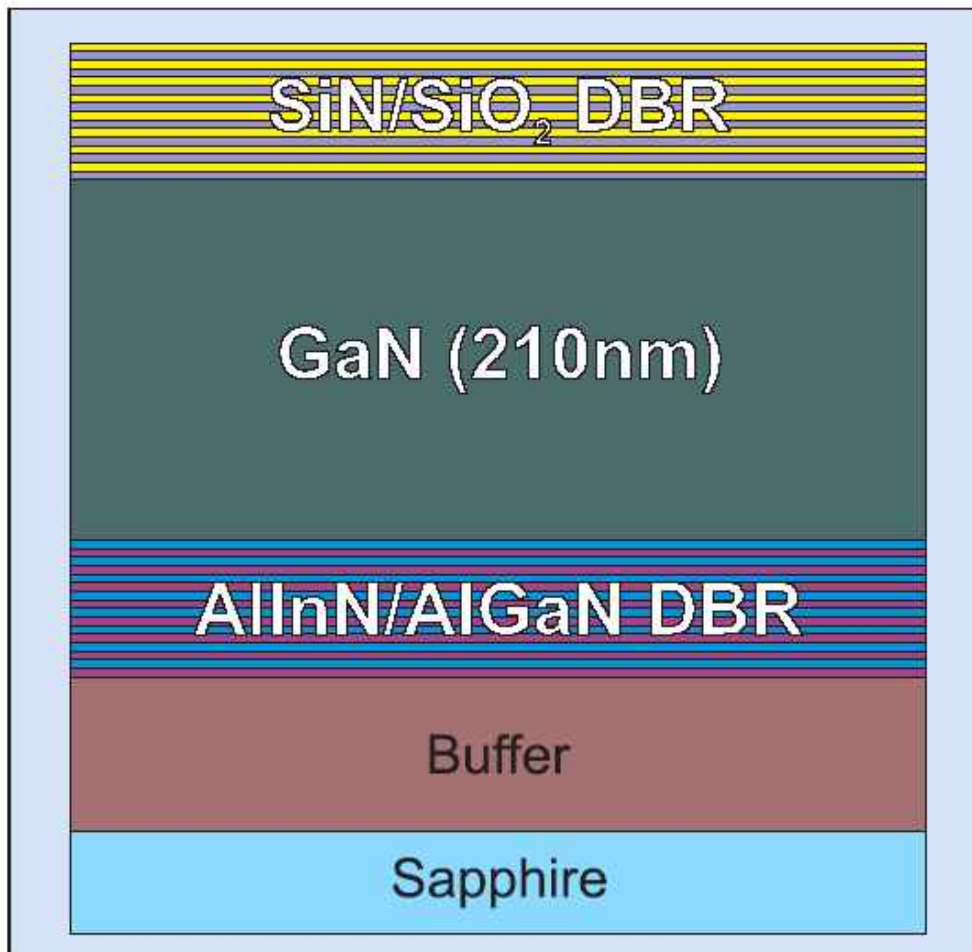
Figure 2. Schematic structure of bulk GaN cavity used to produce polariton lasing.
