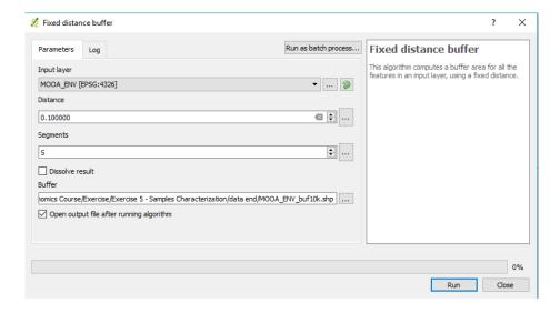
Set MOOA\_ENV as Input Layer, and 0.1 as distance (it represents 0.1 of the project reference system unit EPSG:4326, *i.e.* 0.1 degree  $\sim$  10 km).
