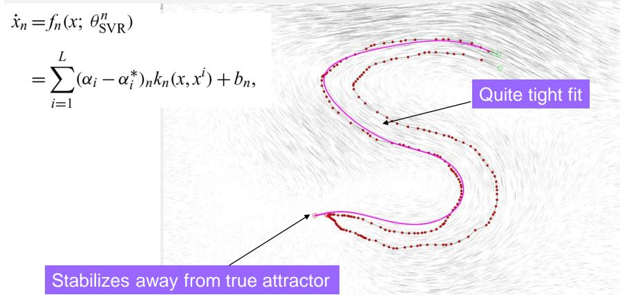
Fit using RBF kernel with tiny  $\varepsilon$  loss and small kernel width.
