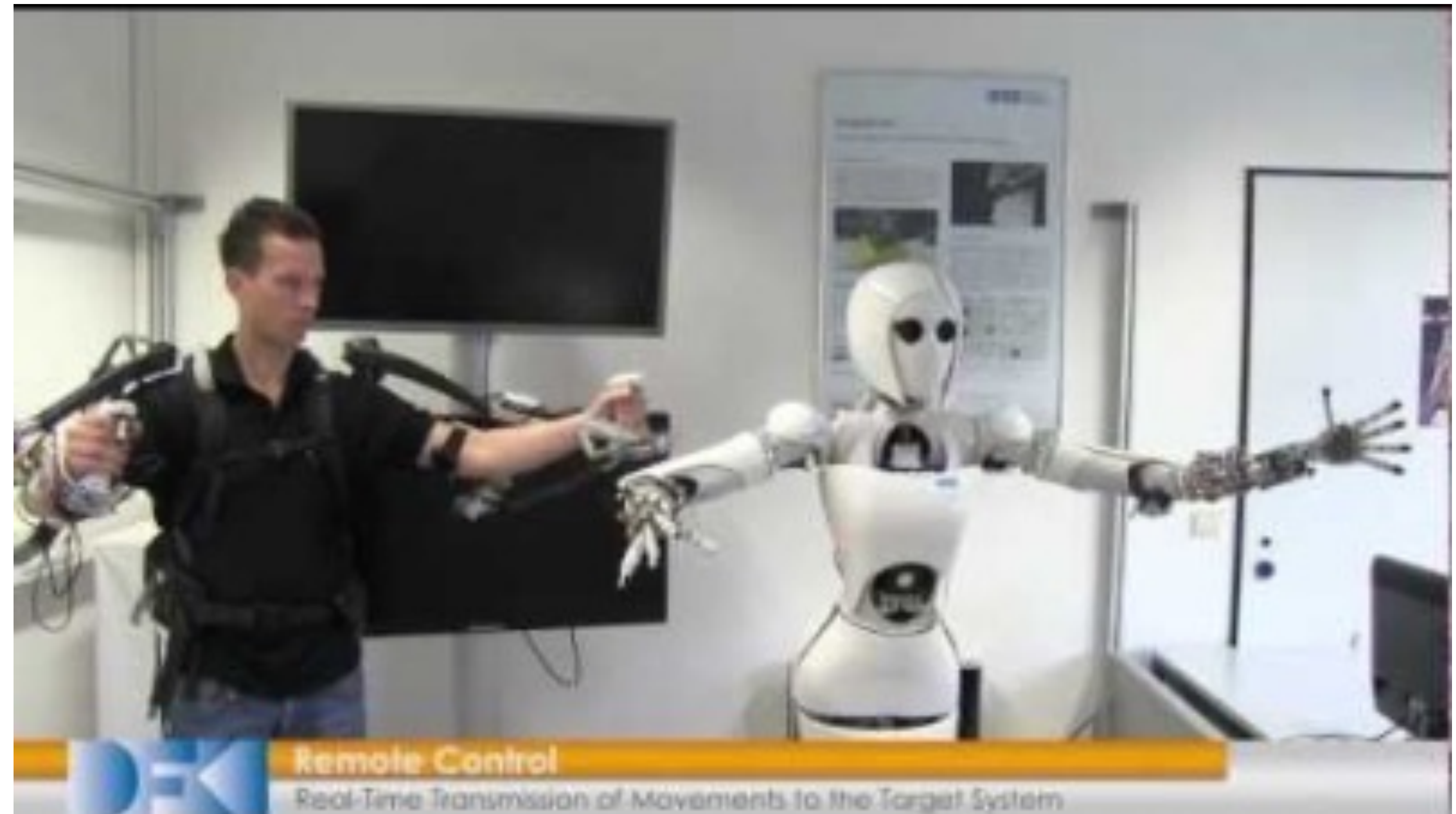
Capio Upper Body Exoskeleton for Teleoperation by the DFKI GmbH Robotics Innovation Center. https://robotik.dfki-bremen.de/en/research/projects/capio.html
