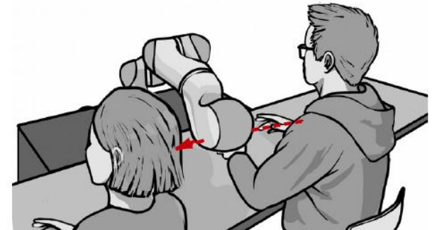
C. Compliant robot: collision risk during change of direction
