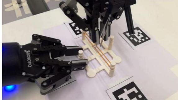
2. Grasp one stick on the board with one robotic arm to stabilize it.
