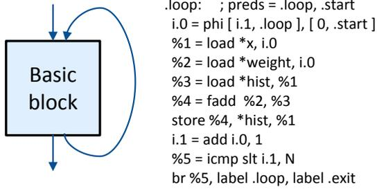
Fig. 2: The histogram kernel from Figure 1, shown as a basic block (left), with a simplified version of the LLVM intermediate representation representing the code (right). This is the starting point for translating the kernel into a dynamically-scheduled circuit.
