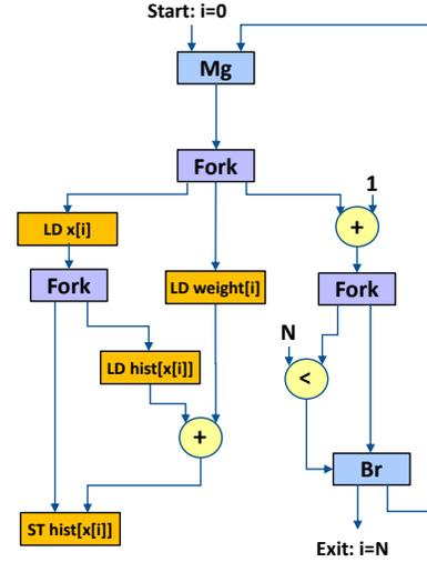
Fig. 3: The histogram kernel translated to an elastic circuit. The basic block body is converted to a dataflow circuit consisting of elastic components. The basic block inputs and outputs employ Merge and Branch nodes to propagate data across basic block boundaries, in accordance with the control flow of the kernel. Fork nodes distribute tokens from one node to multiple successors.
