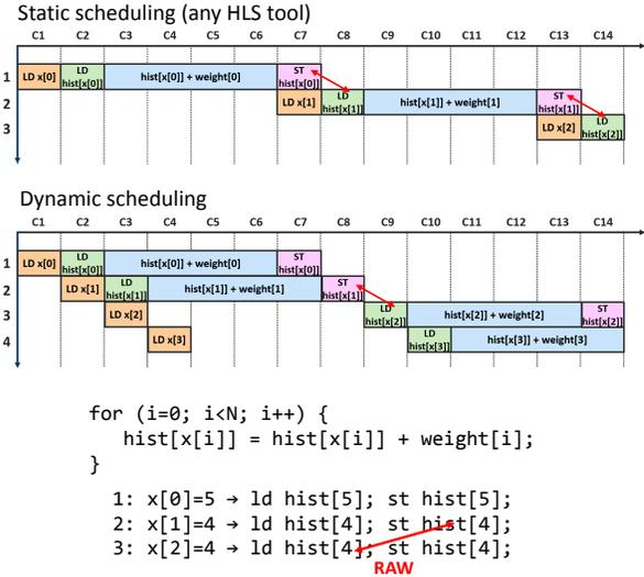
Fig. 1: A static schedule produced by a standard high-level synthesis tool, compared to a dynamic schedule generated by our approach. The HLS tool conservatively assumes that a dependency exists between each pair of loop iterations, whereas the dynamic design only stalls when dependencies occur (in this case, between iterations 2 and 3).
