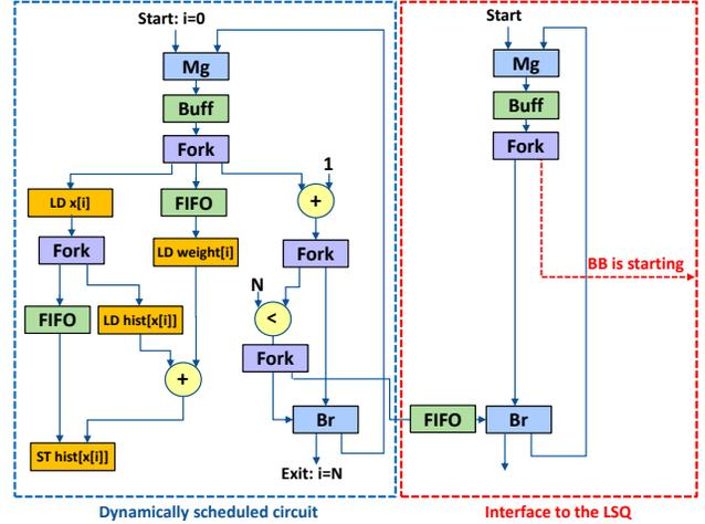
Fig. 7: A dynamically-scheduled elastic implementation of the histogram kernel (left). The LSQ interface (right) notifies the LSQ to allocate entries when control is transferred to a new basic block. The LSQ uses this information to correctly handle memory dependencies.
