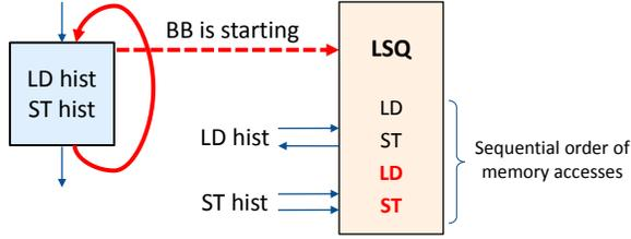
Fig. 6: An LSQ with an allocation policy designed for dynamically scheduled circuits [17]. When the program transfers control from one group (i.e., basic block) to another, the LSQ allocates all memory accesses that the group will generate. In the example from Figure 1, group allocation includes one read and one write per iteration, enabling the LSQ to handle out-of-order memory requests.
