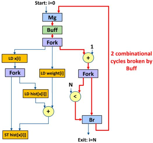
Fig. 4: Elastic buffer insertion to break combinational loops.
