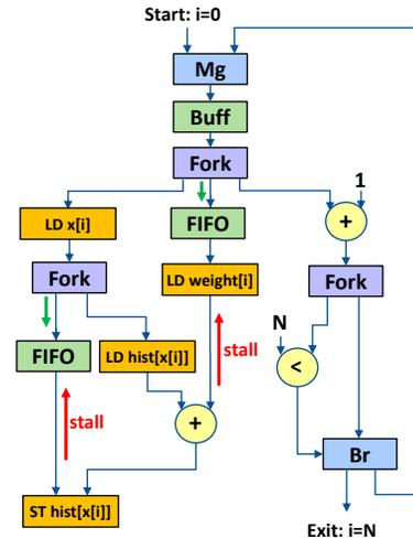
Fig. 5: Inserting FIFOs on Fork outputs can reduce backpressure caused by slow paths, resulting in increased throughput.
