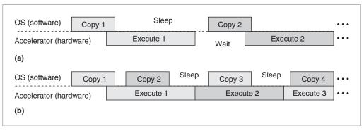
Figure 13. Execution timelines of software (OS) and hardware accelerator events without (a) and with (b) dynamic prefetching. In the prefetching case, the virtualization layer (in the OS) uses some idle time to try predicting future memory accesses and speculatively supplying data in advance. This can provide uninterrupted execution of hardware accelerators.
