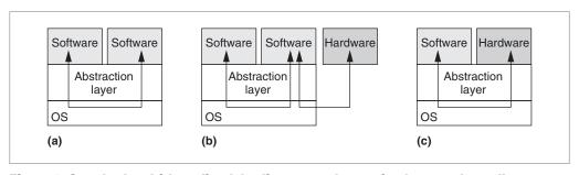
Figure 5. Standard multithreading (a) relies on an abstraction layer and usually some OS services. If the application includes a hardware accelerator (b), there is no systematic support. Instead, the programmer must use a wrapper thread. Extended multithreading (c) includes support for hardware accelerators in the abstraction layer and the OS, permitting seamless integration of software and hardware.
