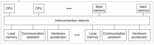
Figure 9. Reconfigurable parallel architecture: Computing nodes (standard processors and hardware accelerators) communicate through a general interconnection network. Hardware accelerators interface to local memories and the rest of the system through standardized communication assistants (CAs).
