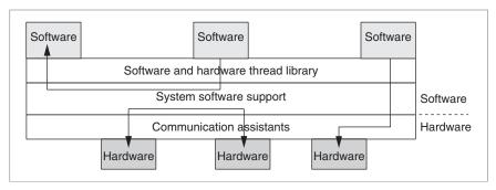
Figure 10. Software and hardware threads connect through the virtualization layer.
