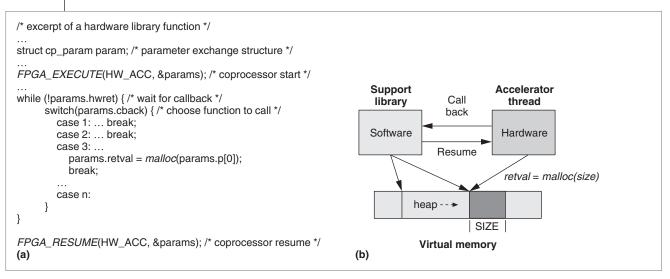
Figure 15. Library code for malloc callback (a). In code execution (b), the accelerator calls back the software. The library code calls the appropriate function, and it passes the returned virtual-memory pointer to the accelerator. Hardware accelerator execution then resumes.
