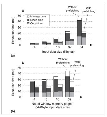
Figure 14. Virtualization layer with and without dynamic prefetching: total execution times of ADPCM for different input data sizes (a); total execution times of IDEA for different numbers of local memory pages (b). Execution time consists of copy time (for transferring data to and from local memory), sleep time (the OS is idle, and the accelerator is possibly processing data), and manage time (for managing VMW data structures).
