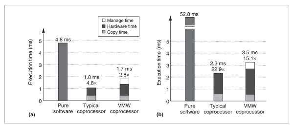
Figure 12. ADPCM (a) and IDEA (b) execution times. Coprocessor execution time consists of copy time (spent in software for transferring data to and from local memory), hardware time (spent in hardware for processing data), and manage time (spent in software for managing system data structures). Input data size is 2 Kbytes for ADPCM and 8 Kbytes for IDEA.
