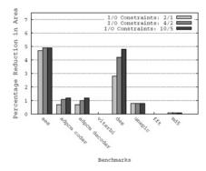
Fig. 18. Percentage reduction in the hardware area of the chosen ISEs without affecting the speedup.
