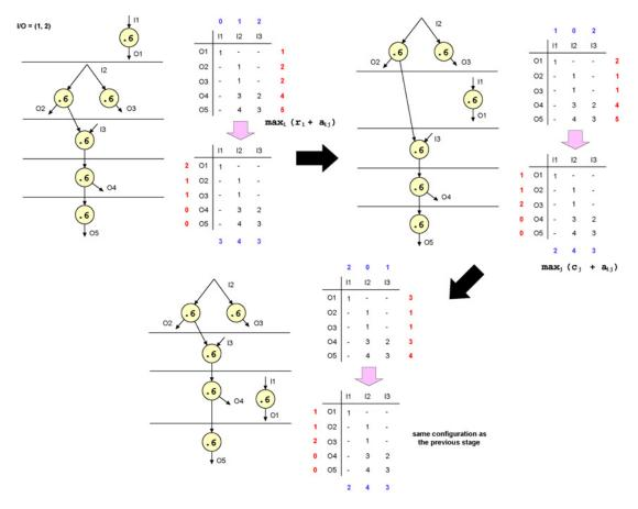
Fig. 12. Execution of the Ping-Pong Algorithm on a simple example; it finds the optimal solution only in two iterations.
