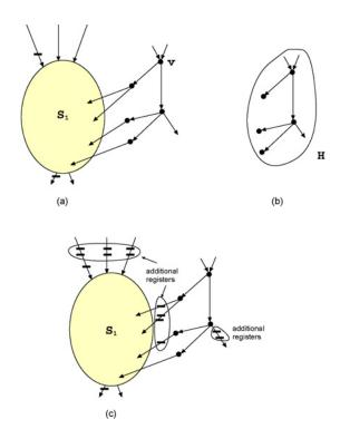
Fig. 6. Adding a single node to a convex subgraph and all paths from this node to the subgraph increases the speedup. (a) Addition of all paths from a node to original subgraph. (b) Graph corresponding to the added node. (c) Resulting ISE after I/O serialization.
