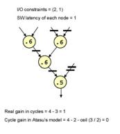
Fig. 4. Example showing that the penalty for I/O accesses is not constant, and can be zero in some cases.
