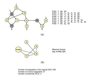
Fig. 10. Example of forming a cluster graph from the original graph and enumerating its maximal cliques. The nodes labeled as  $x_i$ 's in the graph indicate forbidden nodes. (a) Original DAG and the consistent set of its nodes. (b) Cluster graph and its maximal cliques.
