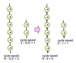
Fig. 2. Example showing that the relative merit of AFUs might change after I/O serialization. The software latency of each node is 1.0.
