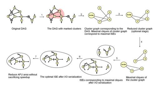
Fig. 3. Summary of our approach to optimal ISE identification and serialization.
