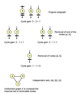
Fig. 14. Example showing that it may be possible to remove two nodes individually without affecting the gain, but not both simultaneously. The I/O constraint is (2, 1).
