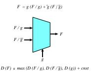
Figure 7: Shannon decomposition with respect to generalized cofactors.
