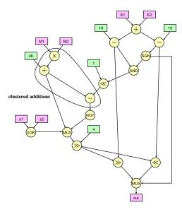
Figure 8: The circuit shown in Fig. 1 can be transformed using arithmetic identities in such a way that the additions and subtractions can be clustered together resulting in a larger compressor tree.
