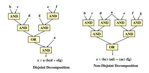
Figure 2: A disjoint decomposition can reduce the number of blocks, but may leave the circuit unbalanced compared to non-disjoint decompositions.
