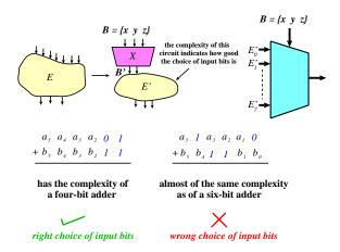
Figure 6: An example illustrating how to decide whether a choice of input bits is right.
