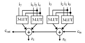
**Fig. 2.** ALM structure in arithmetic mode. The 3-LUTs with shared inputs can be configured as 2-LUTs with non-shared inputs.
