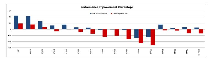
Fig. 9. The percentage of performance gain of non-pipelined radix-4 and *Altera* soft multipliers over non-pipelined *Altera* embedded multipliers.
