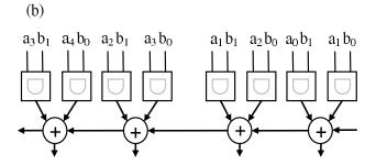
**Fig. 3**. (a) Each two adjacent PPGs can be merged and each two corresponding bits can be fit into an ALM with a required bandwidth of five. (b) Logic cell level representation of two merged PPGs.
