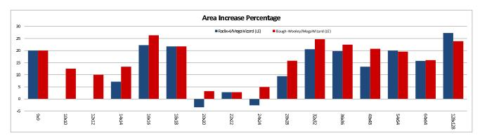
**Fig. 8**. The percentage of area (LAB) overhead of non-pipelined radix-4 and Baugh-Wooley soft multipliers over non-pipelined *Altera* soft multipliers.
