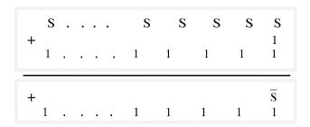
**Fig. 4**. Reducing the repetitive sign bits by adding with  $\pm 1$ .
