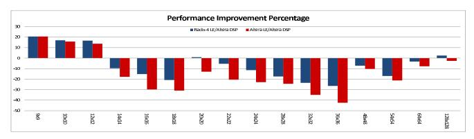
**Fig. 10**. The percentage of performance gain of 1-stage pipelined radix-4 and *Altera* soft multipliers over 1-stage pipelined *Altera* embedded multipliers.
