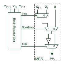
**Fig. 1**. Radix-4 Booth PPG unit. Each PPG output bit is a 5-input function, which has two shared bits with the previous/next PPG function.
