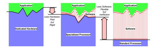
Figure 1: Specialising a processor might achieve the optimal compromise between speed and power design goals and flexibility.
