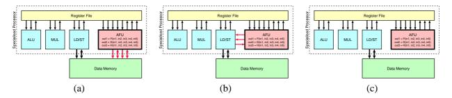
Figure 3: Processor with five-input three-output ad-hoc functional unit. (a) Direct interface with arbitrary bandwidth between Data Memory and AFU. (b) Interface via Load/Store unit and one transaction per cycle between Data Memory and AFU. (c) No interface between Data Memory and AFU.
