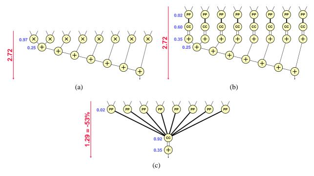
Figure 11: Slightly simplified main subgraph of both dominant mpeg2decode basic blocks before and after arithmetic transformations: (a) original subgraph; (b) actual implementation using partial product generators (PP), column compressors (CC), and carry-propagate adders; (c) optimised implementation, more than twice faster. The numbers indicate the relative delay  $\Lambda_{\rm hw}$  and the critical path delay  ${\rm CP_{hw}}$ .
