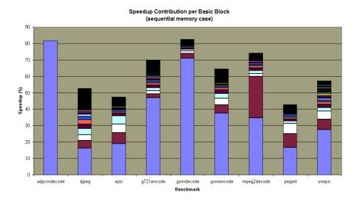
Figure 9: Speedup contribution per basic block after ILP transformations in the case of sequential memory accesses. Note that now to achieve approximately  $1.5 \times$  speedup, only a single AFU suffices in most cases.
