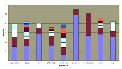
Figure 5: Speedup achievable by mapping the most important basic blocks on AFUs. Note that to achieve approximately  $1.5 \times$  speedup, only 2–3 AFUs are needed in most cases, and 5–6 at worst.
