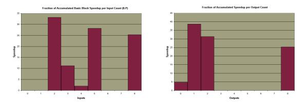
Figure 10: Histograms of the potential speedup per input and output count, after ILP transformations. Compared to Figure 4 multiple register-file writes are slightly reduced and the importance of several reads increased.
