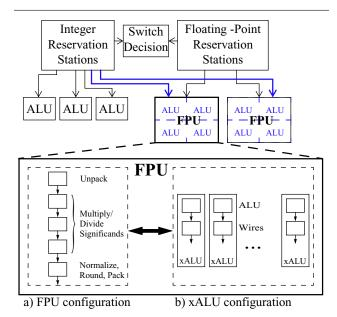
Figure 1. Paths between reservation stations and functional units (top), and reallocation possibilities (bottom). Each FPU can be reallocated as a number of *extra ALUs* (*xALUs*). FPU operations have 5 stages, the *xALUs* have 2 stages, all of which must be idle to allow reallocation.
