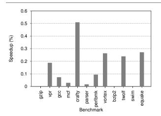
Figure 8. Speedups of *balance* over *threshold*, run on the *mainstream* model. In these benchmarks, *balance* is always the same or better than *threshold*, but with an average gain of only 0.14%. The others (not shown) have negative speedups due to very fast changes in the instruction type distribution and the rounding of r(k).
