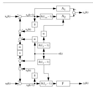
Figure 3. Decision Problem. m and n are the number of ALUs, resp. FPUs.  $\alpha$  is the number of xALUs per FPU,  $A_1$  and  $A_2$  are the left and right parts of the sum in equation (3), and F is the right part of equation (4).  $L_{xa}$  and  $L_f$  are the latencies of an xALU and an FPU, resp., and  $\delta(t)$  represents a delay of t cycles.
