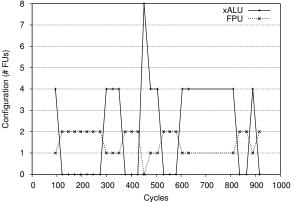
Figure 7. Instruction types (left) and configuration decision (right) for part of the *sixtrack* benchmark. The configuration adapts to the instruction types: when there are few FP instructions, the FPUs are reconfigured as *xALUs*.
