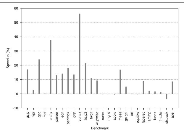
Figure 5. Speedups between the *baseline mainstream* and the *dynamic mainstream* models. The integer benchmarks show universal gains, whereas the FP benchmark results are more varied. All negative speedups are small, less than 0.5% slower than the *baseline*, except for *sixtrack*, with a loss of 3.8%.
