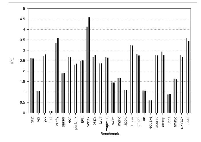
Figure 6. Simulation results for the SPEC benchmarks for the *baseline top* model (light) and *dynamic top* model (dark). The results are usually quite close, with some benchmarks showing larger differences in either direction. The overall average is a tiny gain of 0.24%
