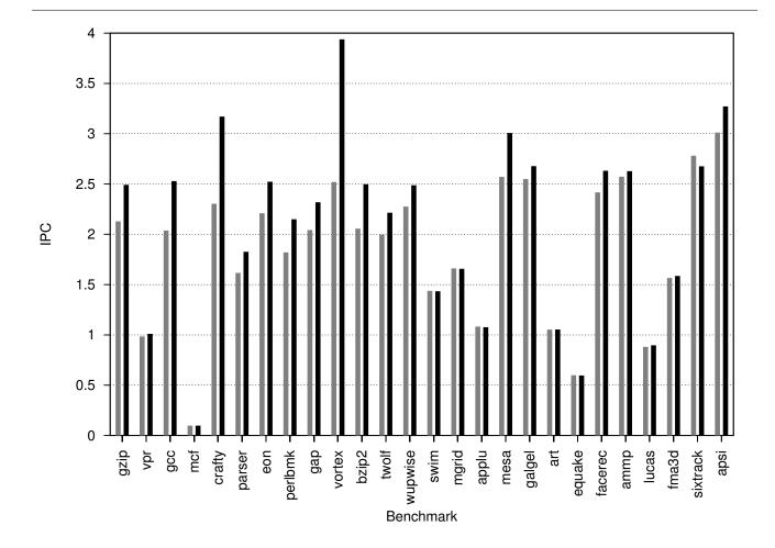
Figure 4. Simulation results for the SPEC benchmarks for the *baseline mainstream* (light) and *dynamic mainstream* (dark) processors. There are large variations in overall IPC, with some significant gains by the *dynamic* model.
