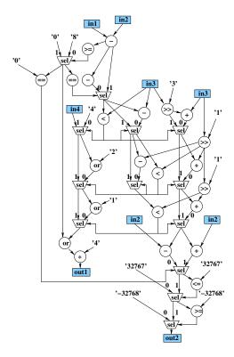
Figure 8: An ISE for ADPCM ENCODER (adpcm-e) having 4 inputs and 2 outputs; each operation node maps to a hardware component.
