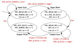
Figure 7: Communication Template for AFU Interface in Microblaze
