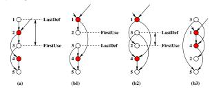
Figure 4: The ISE here is composed of the shaded instruction nodes. (a) An example showing the *LastDef* point and the *FirstUse* point; (b1) an example where it is not possible to insert the ISE under consideration; (b2) After code restructuring; (b3) positioning of the ISE between *LastDef* and *FirstUse*.
