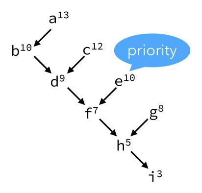
A node's priority is the length of the longest latency-weighted path from it to a root of the dependence graph
