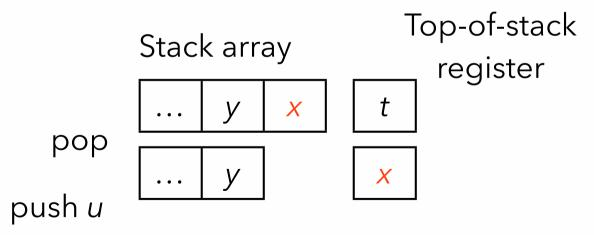
In a stack-based VM, the stack is typically represented as an array in memory. Since almost all instructions access the stack, it can be interesting to store some of its topmost elements in registers.
