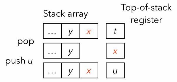
In a stack-based VM, the stack is typically represented as an array in memory. Since almost all instructions access the stack, it can be interesting to store some of its topmost elements in registers.
