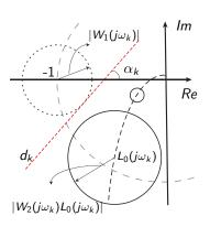
• Performance circle replaced by a tangential  $d_k$  line with angle  $\alpha_k$ :
