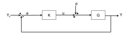
Given that  $G(0) = \frac{7}{3}$ ,  $Y_c(s) = 0$  and the disturbance d is a unit step, calculate the steady-state error  $e(\infty)$  as a function of K.
