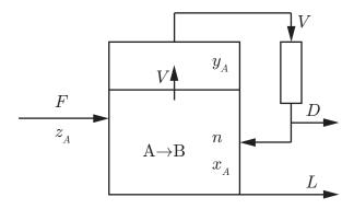
Write the dynamic model for this vessel using n and  $x_A$  as state variables.
