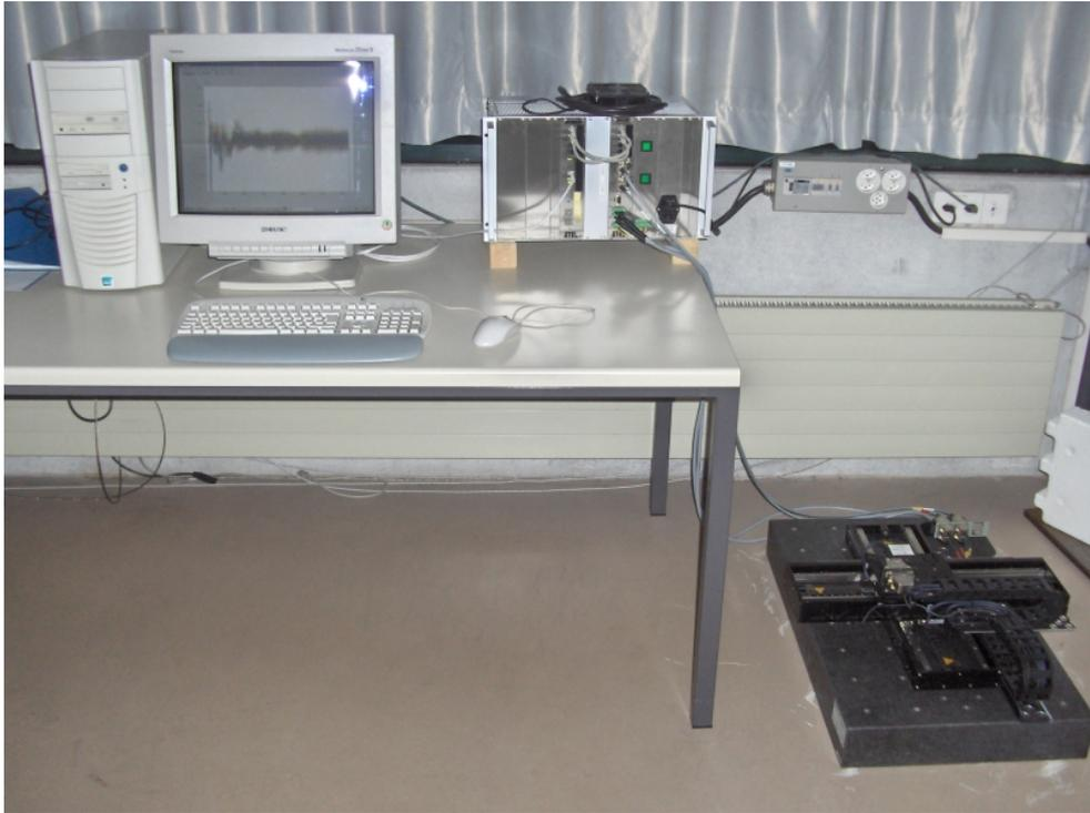
Figure 5.6: Set up used for our experiments: PC (Matlab), Motion Controller and the Linear Motor System (ETEL)
