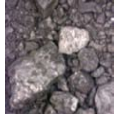
Figure 1: An image from a computer vision system on a coal conveyor is automatically processed to estimate the proportion of fines in the coal.
