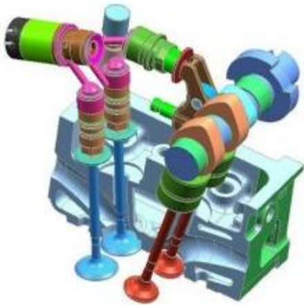
Figure 1. Fiat VVA valve opening schematic (MultiAir).
