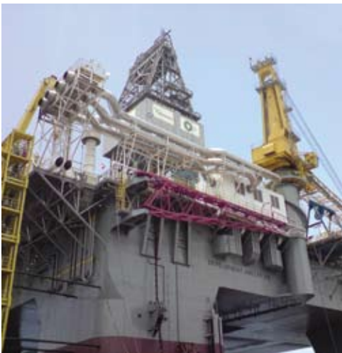
Development Driller III: Fifth generation, dynamic positioning semi-submersible ultra-deepwater drilling rig build by Keppel FELS Singapore.
