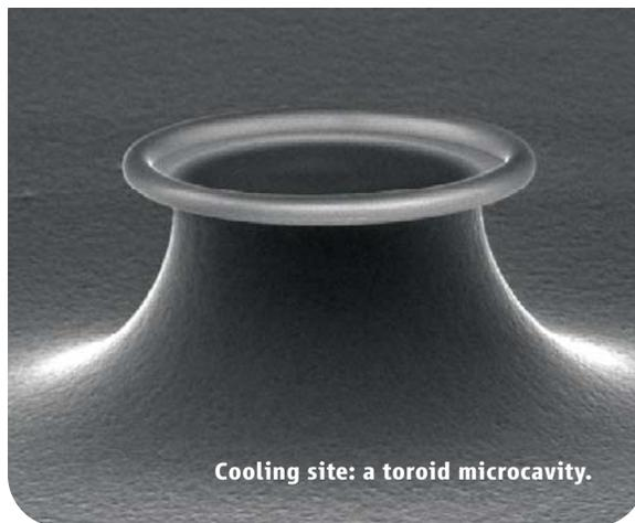
Cooling site: a toroid microcavity.
