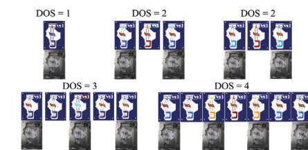
Figure 4. Stable configuration of the T-mechanism for different programming inputs.
