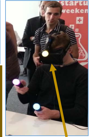
Tracked Oculus HMD with Move controller
