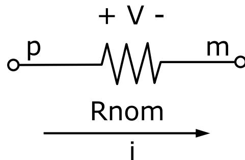
The voltage across this device is determined by the simulator. The current through it is defined by the device characteristic equation:
