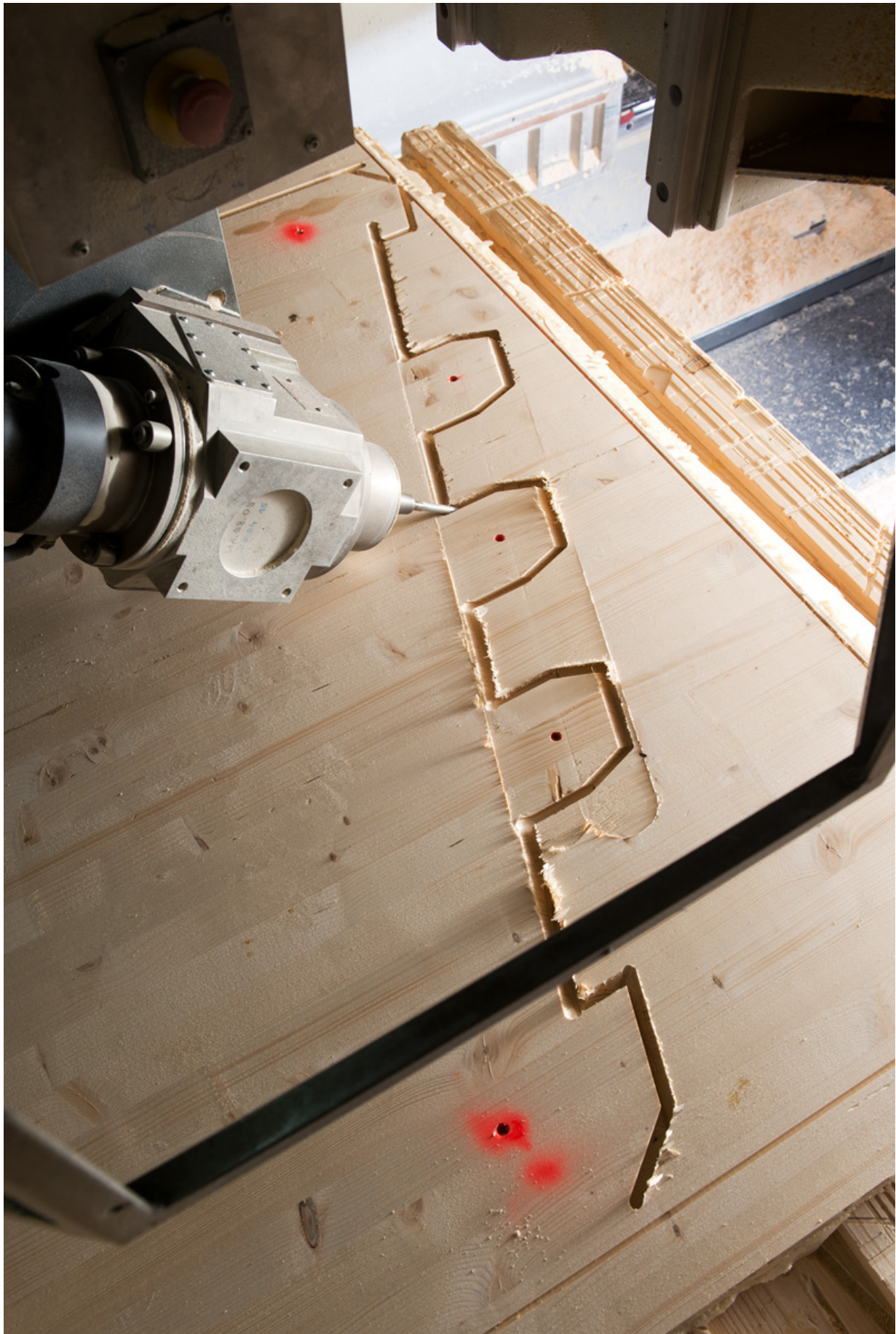
Figure 6. Cutting of the 45mm thick panels (credits: I. Kramer)
