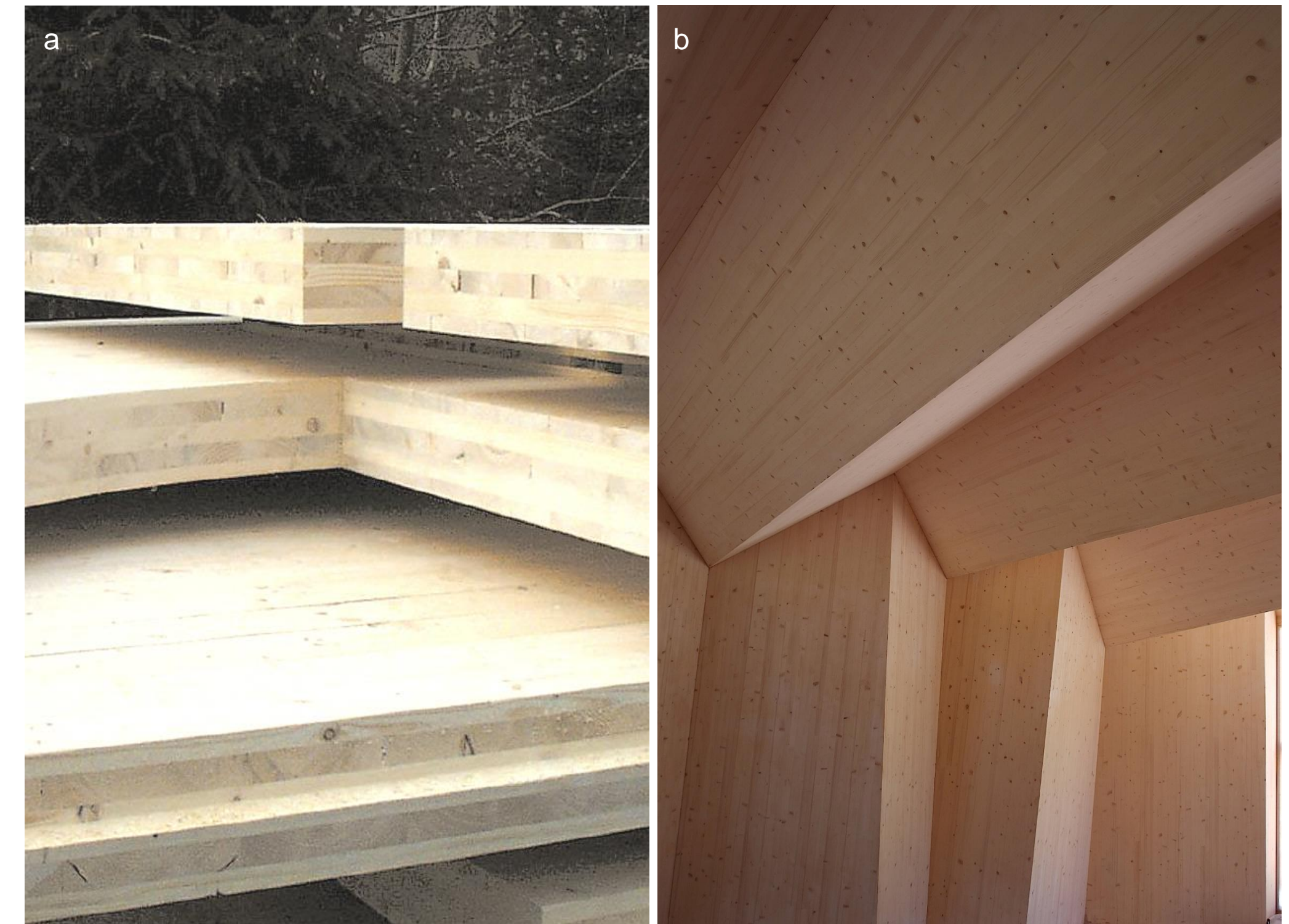
Fig. 2: Samples of glued CLT panels based on U-adhesives (a) and possible assembling of CLT panels to a folded structure (b).
