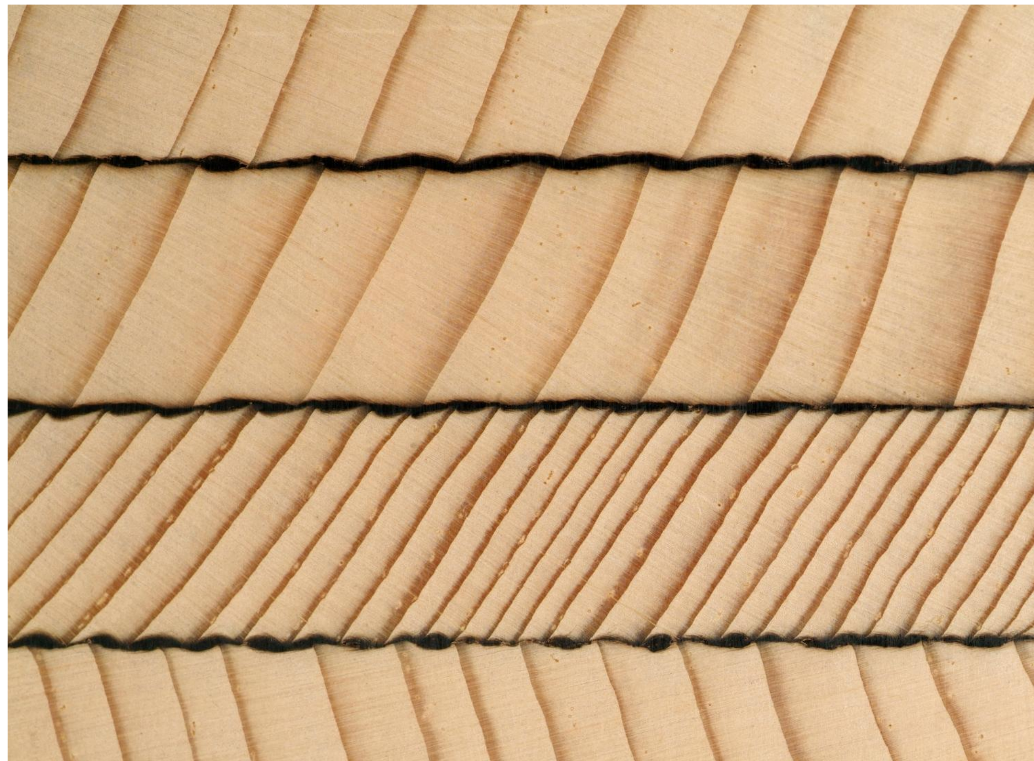
Fig. 1: Zoom on friction welded layers of spruce boards including the distinctive black weld line.
