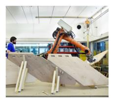
Bespoke Digital Prefabrication augments the advantages of manufacturing through the use of digital building technologies. It enables custom-designed, large-scale digital prefabrication of complex architectural elements. Researchers work at the 1:1 building scale, developing resource-efficient material systems, joining methods, design tools and computational technologies.
