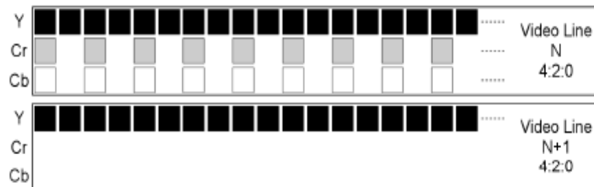
Figure 1-5 4:2:0 YCbCr Sampling format
