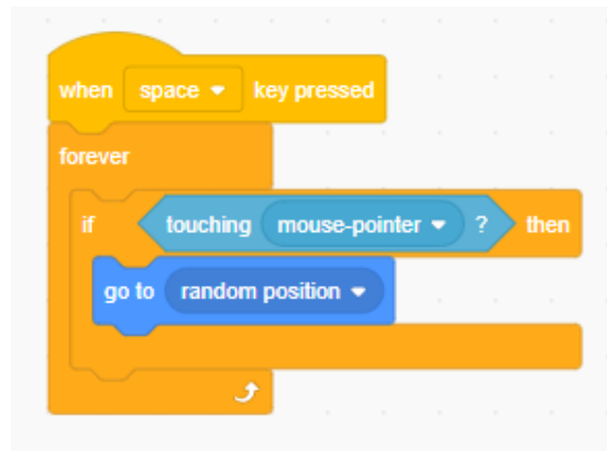
Figure 2.2 – A simple Scratch program that repeatedly checks if the mouse pointer is touching the cartoon sprite and moves it to a random position if so.
