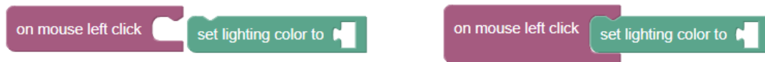
Figure 6.8 – In terms of sizes, the socket of the ‘on mouse left click’ block is smaller in height than the height of the ‘set lighting color to’ block. Yet, when the latter is fit into the former, the height of the socket changes to accommodate the incoming block.
