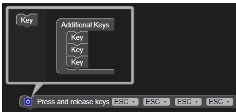
Figure 7.8 – The implemented mutator allows appending any number of additional key input fields to the block by stacking the same number of 'keys' blocks inside the 'Additional keys' block.
