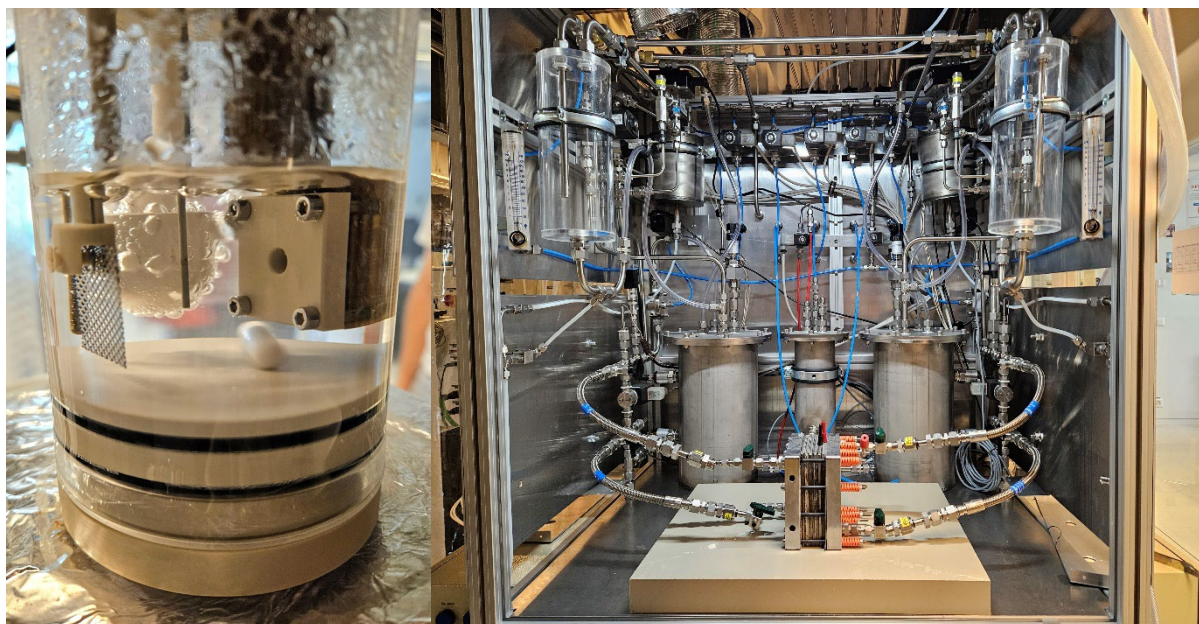
Figure 1: a) 3-electrode system for conducting AST b) Real experimental AEMWE cell stack
