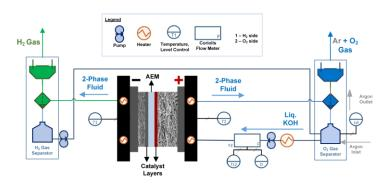
Figure 1: a) scheme of AEM stack with a simplified BoP.
