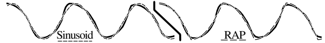
FIG. 1. The experimental crack path used in Ref. [1] (solid curve) is fitted by our two reference models (dashed curves). Both fits are significantly better than the one obtained by the authors with their cycloidal construction, as revealed by comparison with Fig. 2(c) of the original Letter [1].
