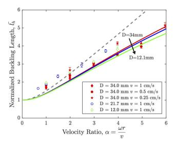
Fig. 3 Normalized buckling length,  $\bar{I}_h$  versus dimensionless rotation speed,  $\alpha$ . The experiments were conducted in the following ranges of parameters:  $12.1 \le D \text{ (mm)} \le 34$ ;  $0.25 \le v \text{ (cm/s)} \le 1$ ; and  $0 \le \omega \text{ (rpm)} \le 300$ . The dashed line represents the simplified theory given by Eq. (7), and the solid lines represent the more sophisticated theory given by Eq. (18).
