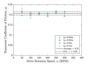
Fig. 7 The transverse friction coefficient,  $\mu_b$  is experimentally found to be independent of the rotation speed,  $\omega$ , and the rod length, I, which is inserted into the constraint. The solid and dashed horizontal lines correspond, respectively, to the average and standard deviation of all the data;  $\mu_t$  = 0.21  $\pm$  0.01.
