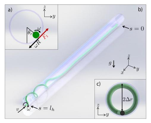
Fig. 1 Schematic definition of the problem. (a) Diagram of transverse forces exerted on the rod during axial rotation. (b) Representation of the helical buckling configuration that occurs when the injected length of the rod is  $I_h$ . (c) Definition of the radial clearance,  $\Delta r$ , between the rod and the constraint.
