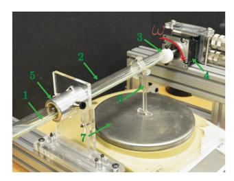
Fig. 6 Apparatus used to measure the transverse friction coefficient,  $\mu_{\rm L}$  A polymeric rod (1) is inserted into a 40 cm length of borosilicate tubing (2) and connected via rod clamp (3) to a servomotor (4) which provides axial rotation. The borosilicate tubing is mounted in a rotary air bushing (5) to allow complete transmission of torque through a tubing-mounted reaction arm (6) to a laboratory scale (7) placed below the apparatus.
