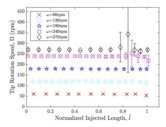
Fig. 4 Rotation speed of the tip,  $\Omega$ , as a function of the dimensionless injected length  $\bar{I}=I/I_h$  (normalized by the helical buckling length  $I_h$ ), for five different values of the drive rotation speed (see legend). Each data point represents an average of  $\Omega$  for five full revolutions, and the error bars are the associated standard deviation. The diameter of the cylindrical constraint was  $D=21.7\,\mathrm{mm}$  and the injection speed was  $v=1\,\mathrm{cm/s}$ .
