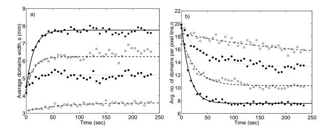
Figure 3. (a) Time-series of the average domain width,  $\phi$ . (b) Time-series for number of domains,  $\eta$ . (c) C=0.873, (e) C=0.729, (o) C=0.708, (o) C=0.602. Lines are fits to Eqn. (2). All runs were started from a homogeneously mixed layer.
