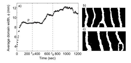
Figure 2. (a) Time series of the average domain width,  $\phi$ , over 20min, for C = 1.057. (b)&(c) Binary frames of the segregation patterns (regions of poppy seeds in black and regions of phosphor-bronze spheres in white) at (b)  $t_A = 300sec$  and (c)  $t_B = 702sec$ .
