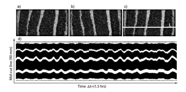
Figure 6. Photographs of the granular layer showing the oscillatory bending of the phosphor-bronze stripes (regions in white), at different times: (a) beginning of cycle, (b) half-cycle, (c) end of cycle. (d) Space time diagram constructed from stacks of the cut line, L in (c), over 1.5hrs.
