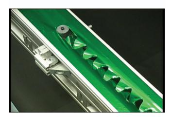
FIG. 1. (Color) Oscillatory fracture paths obtained when cutting a thin polymer sheet (mylar) with a blunt cylindrical cutting tool (36 mm diameter) (enhanced online).
