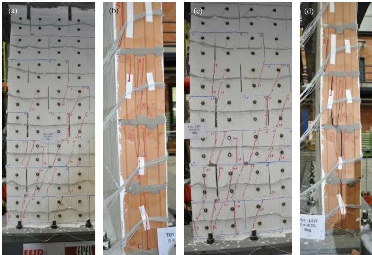
Figure 12: Crack pattern at LS27 ( \delta = -0.3\% ) of the compressed corner of the first storey of the URM wall. Before (a, b) and after (c, d) the horizontal load failure.
