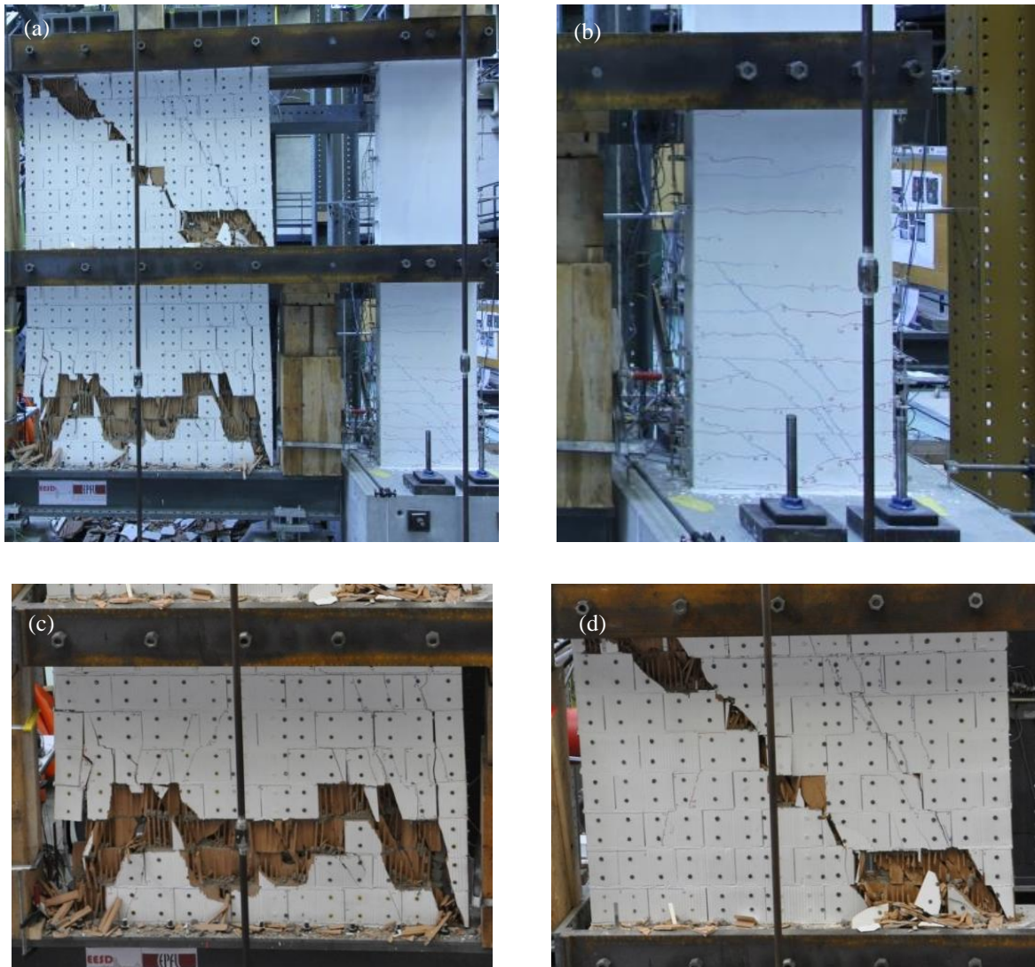
Figure 14: Crack pattern at LS33, \delta = +0.95\% . (a) specimen; (b) RC wall, first storey; (c, d) close-ups of the first and second storey of the URM wall.
