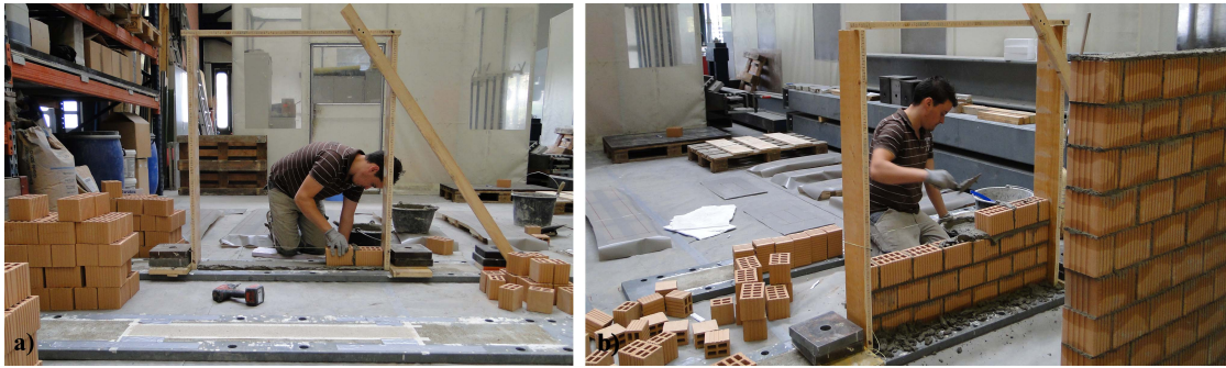
Figure 2 Steel plates with layer of quartz sand and test units during construction
