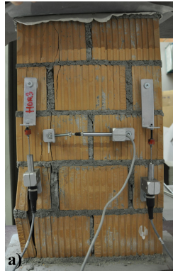
Figure 4 (a) Specimen for the compression tests with mounted measurement devices and (b) stress-strain relationships
