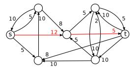
The residual network after augmentation looks as follows. The next augmenting path is marked red. We can augment 5 units of flow.
