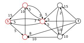
There is no more s-t-path in the residual network. Thus our flow is maximal and of value 20. The nodes marked red are reachable from s. Thus  $\{s, u, v, x\}$  defines a minimal s-t-cut. The flow is as follows:
