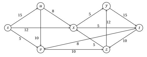
Run the Ford-Fulkerson algorithm to compute a max s - t-flow. For each iteration give the residual network and mark the path you choose for augmentation.
