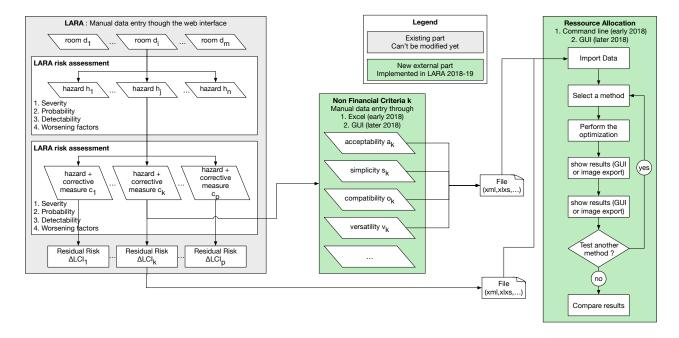
Figure 1: The intended work flow of the project. The part in grey shows the existing functionality of LARA.
