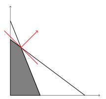
The optimal solution is at the intersection of two of the constraints set to equality, so it is the solution to the system of linear equations:
