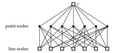
From the properties of the Fano plane we see that each node (except of the root) has degree 4. If we install capacities of 1/4 on each edge (directed upwards), then clearly the solution is feasible
