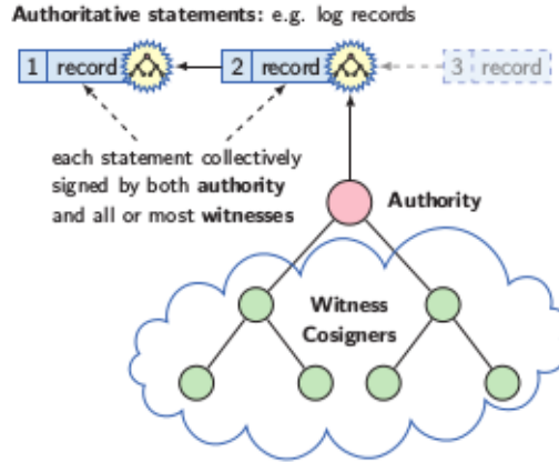
Figure 1: ByzCoin’s collective signing protocol: The nodes are organized in a tree structure and collectively sign each block (copied from [15]).
