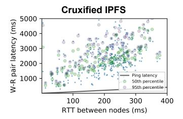
Average of Write + Read pair latency in ms according to the RTT between the nodes
