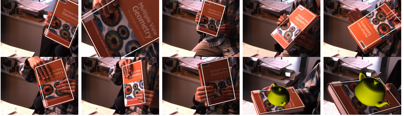
Fig. 1. Detection of a book in a video sequence: As shown by the white outline, the book is detected independently and successfully in all frames at 25Hz in 640 \times 480 images on a standard PC, in spite of partial occlusion, cluttered background, motion blur, large illumination and pose changes. In the last two frames, we add the inevitable virtual teapot to show we also recover 3-D pose.
