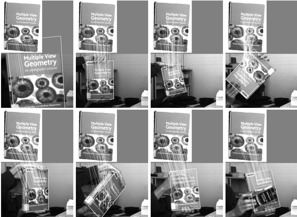
Fig. 15. Detection of the book: The white lines represent the inlier matches established in real-time under several poses.
